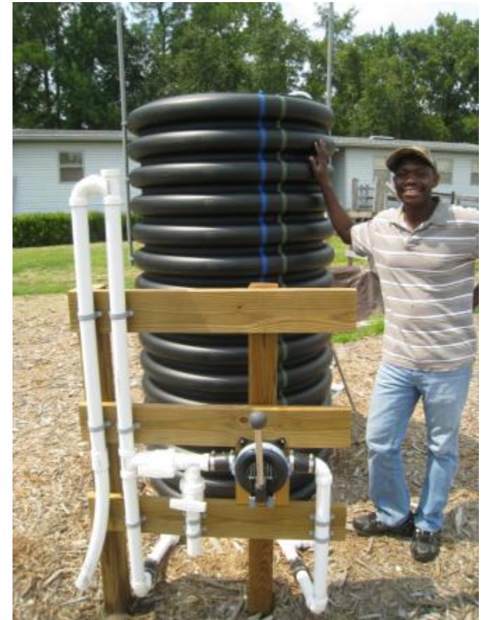
Anaerobic digester appropriate for Haitian rural areas
